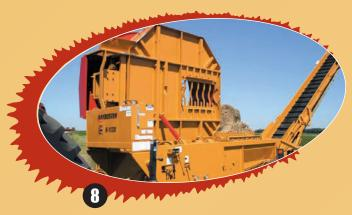
9. The 21' (6.4 m) long x 24" (60.96 cm) wide hydraulicallyfolding conveyor is designed for the increased capacity of a 10' tub grinder. The conveyor folds over the top of the tub for easy transport. It is capable of stacking material up to 14' 9" (4.5 m) high at a 40 degree angle.
